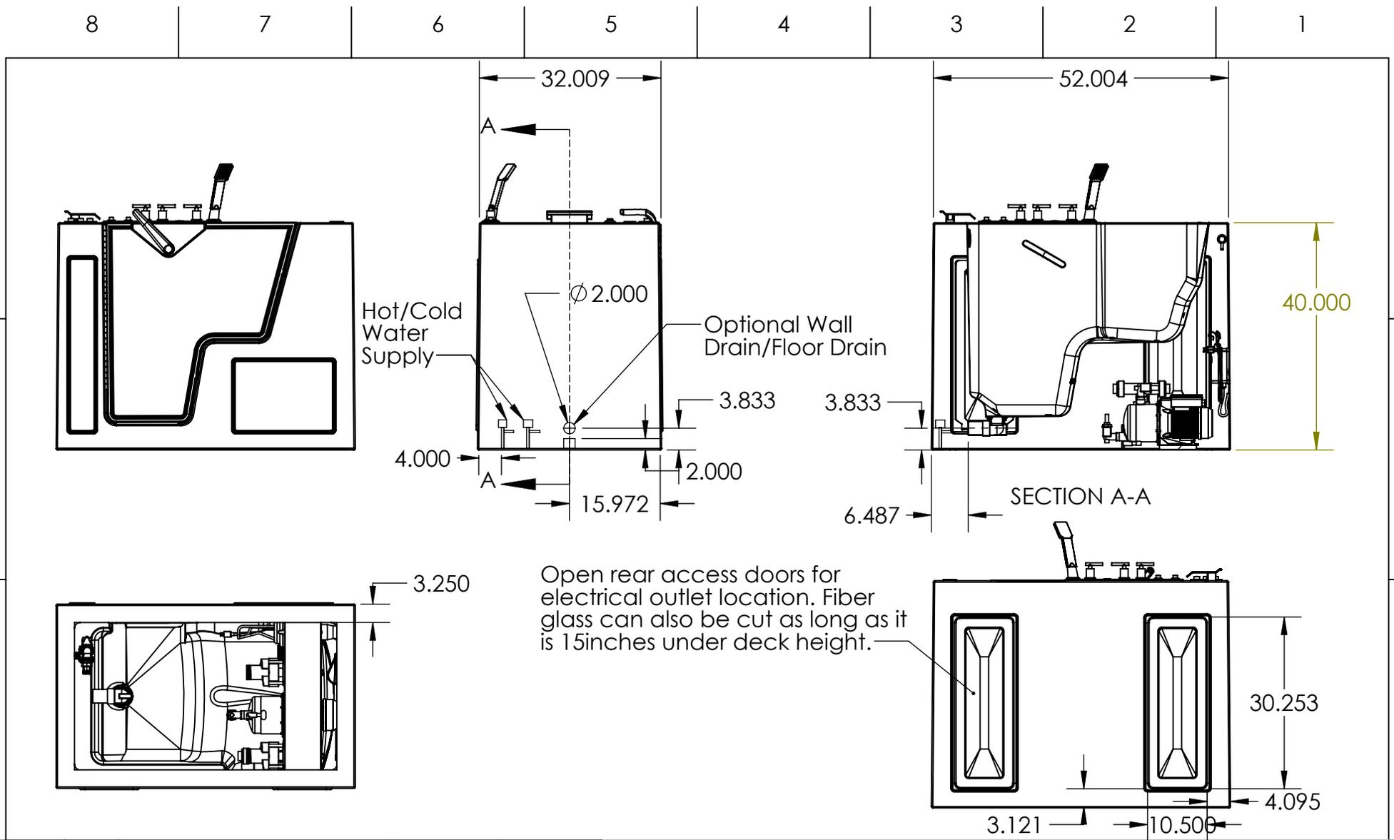
Open rear access doors for electrical outlet location. Fiber glass can also be cut as long as it is 15 inches under deck height.
