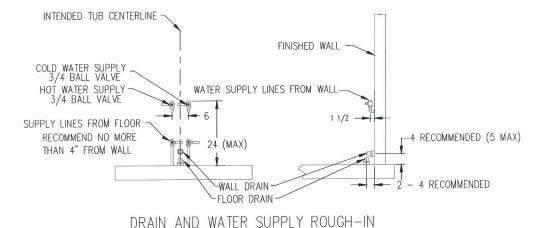
TUB IS EQUIPPED WITH A FLEXIBLE DRAIN TUBE WITH A CUFF THAT FITS OVER A 1 1/2" DIAMETER DRAIN PIPE. (HOSE CLAMP FOR CUFF IS SUPPLIED) DRAIN REQUIREMENT: MINIMUM OF 1 1/2" (NOMINAL) PVC TUBE WITH SLIP ADAPTER FOR 1 1/2" DIAMETER EXTENSION TUBE. THE EXTENSION TUBE TO BE EXPOSED AT MINIMUM 1 1/2" FOR CUFF ATTACHMENT.
