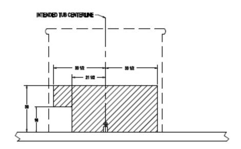
HATCHED AREA IS OPEN WALL SPACE BEHIND THE CABINET (EXCEPT FOR DRAIN CONNECTION)
