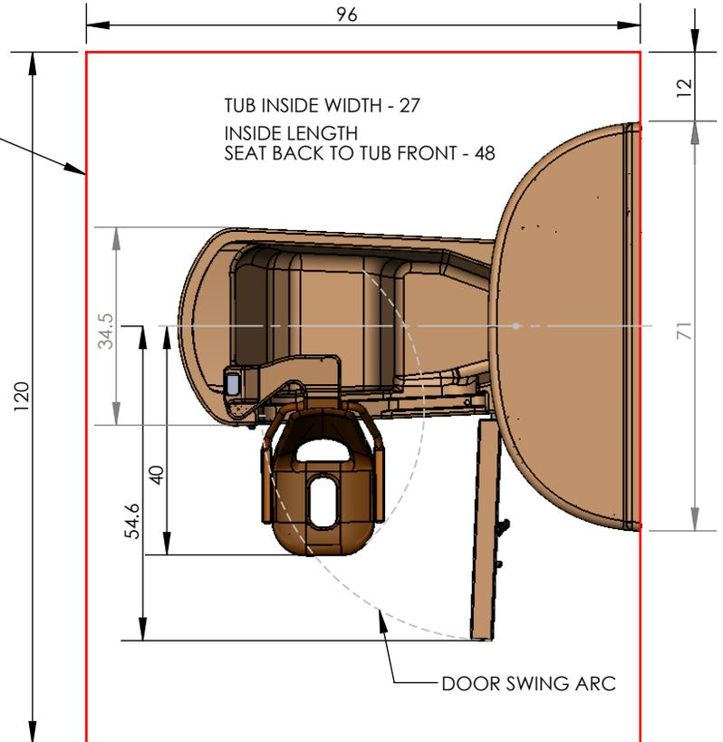
TO TRANSPORT THIS TUB INTO A ROOM, THE DOOR OPENING WIDTH MUST BE 35 INCHES MINIMUM.
