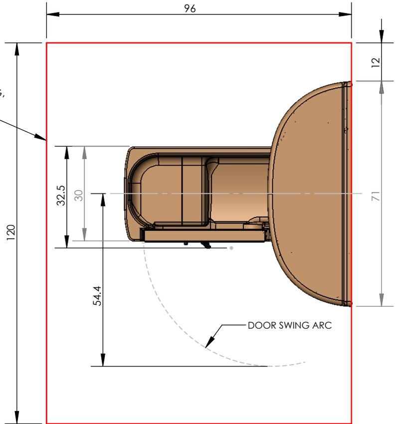
TO TRANSPORT THIS TUB INTO A ROOM, THE DOOR OPENING WIDTH MUST BE 33 INCHES. HOWEVER, IT CAN BE AS SMALL AS 30 INCHES IF THE WATER DOOR IS REMOVED FROM THE TUB PRIOR TO ENTRY.
