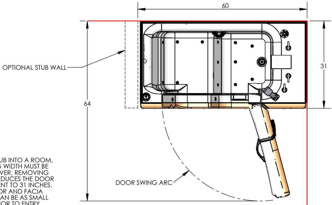
TO TRANSPORT THIS TUB INTO A ROOM, THE DOOR OPENING WIDTH MUST BE 32.5 INCHES. HOWEVER, REMOVING THE DOOR HANDLE REDUCES THE DOOR OPENING REQUIREMENT TO 31 INCHES. IF THE WATER DOOR AND FACIA ARE REMOVED, IT CAN BE AS SMALL AS 29 INCHES PRIOR TO ENTRY.
