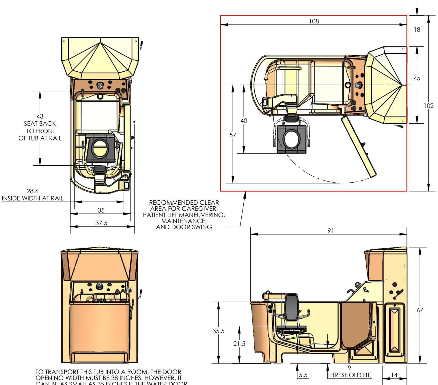
TO TRANSPORT THIS TUB INTO A ROOM, THE DOOR OPENING WIDTH MUST BE 38 INCHES. HOWEVER, IT CAN BE AS SMALL AS 35 INCHES IF THE WATER DOOR AND SHOWER ELBOW ARE REMOVED FROM THE TUB PRIOR TO ENTRY.
