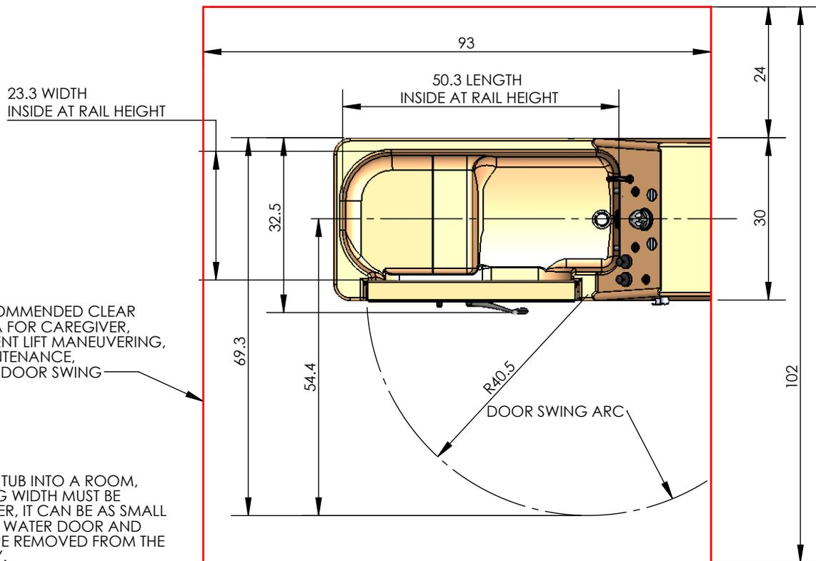
TO TRANSPORT THIS TUB INTO A ROOM, THE DOOR OPENING WIDTH MUST BE 33 INCHES. HOWEVER, IT CAN BE AS SMALL AS 30 INCHES IF THE WATER DOOR AND SHOWER ELBOW ARE REMOVED FROM THE TUB PRIOR TO ENTRY.
